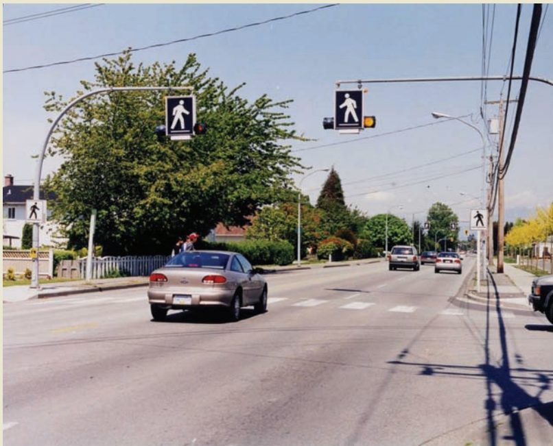
Figure 39: Although not mentioned in the MUTCD, pedestrian activated flashing crosswalks perform similarly to the HAWK signal, but do not require the driver to come to a complete stop. Instead, this form of signal prompts drivers to yield until pedestrians have cleared the crosswalk.
