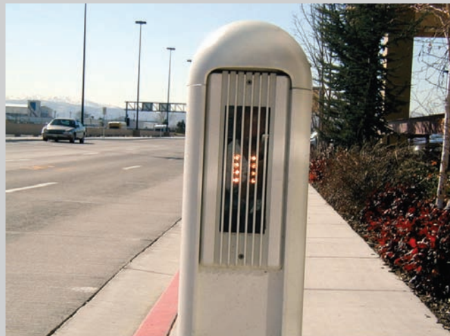
Figure 52: Pedestrian detection devices, such as this, have sensors that detect when a pedestrian is approaching a crosswalk and set off in-pavement lights to flash until the pedestrian has crossed to the other side of the roadway.
