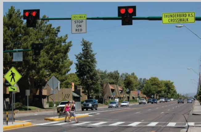
Figure 51: Typical HAWK system with an additional strong yellow-green sign to indicate that this is a high school crosswalk.
