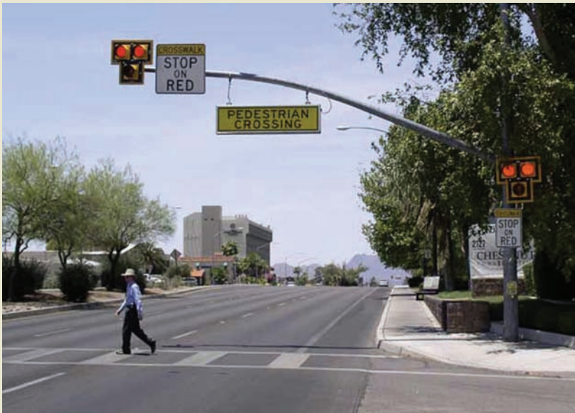
Figure 38: This HAWK signal provides a solid red signal, presenting a clear regulatory message to drivers, resulting in a uniform stop response in lieu of drivers yielding or speeding through the signal to avoid slowing for pedestrians.
