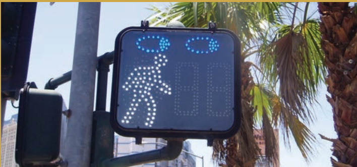
Figure 48: Electronic signs with “animated eyes” in Las Vegas, Nevada remind pedestrians to look for turning vehicles.
